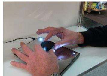
**IMPORTANT NOTICE** - the electronics inside the base may heat up. This may cause that some or all LEDs will turn off, or just make the balancing more difficult. So, if you were unable to balance the magnet after 30 seconds - take a rest for at least 30 seconds to let the electronics cool down. If all LEDs turn off - just unplug the AC adapter, wait for 1-2 minutes, and then plug it back to the mains.
